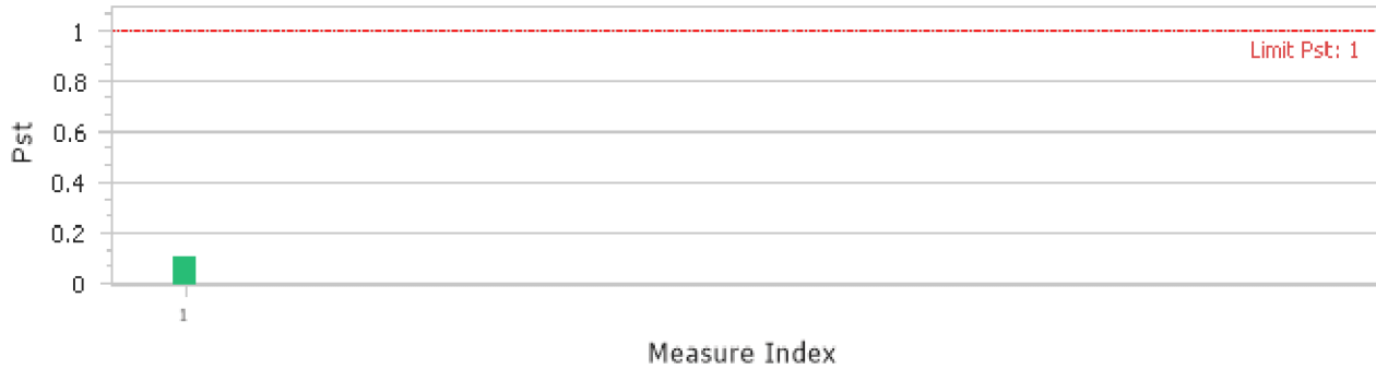
Short-term Flicker Severity (Pst) (Line 1)
