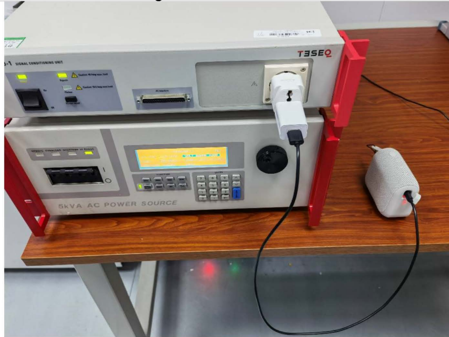
Voltage Fluctuations and Flicker
