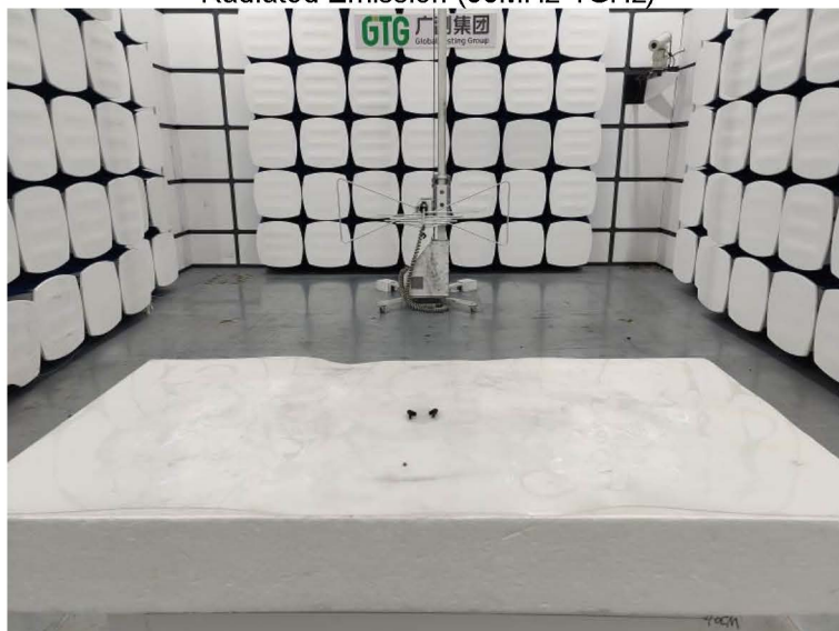
Radiated Emission (1GHz-6GHz)
